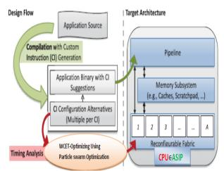
Fig. 1: Tool Flow Performing WCET-Optimizing Instruction Set Selection Integrated with Timing Analysis.
